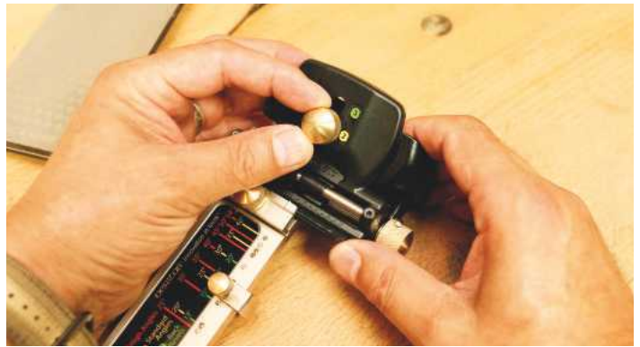
▲ You adjust the body to correspond with the colour setting chosen on the jig
